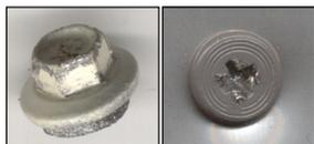
Worn out drive bits and sockets produces poor drilling, can strip the recess, and damage painted fasteners.
