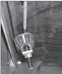
*"...Triangle Fastener's hillside anchors having ridges, serration, on the curvature of the standard hillside washer with Stress-Lok washers were found to be superior to the standard off-the-self market available hillside washers."*
